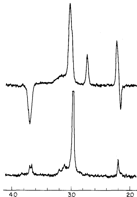
Figure 2. ^1\text{H} NMR spectrum (90 MHz) of p -methylbenzyl benzyl ketone in an aqueous solution containing hexadecyltrimethylammonium chloride in the dark (bottom) and during UV irradiation (top).
